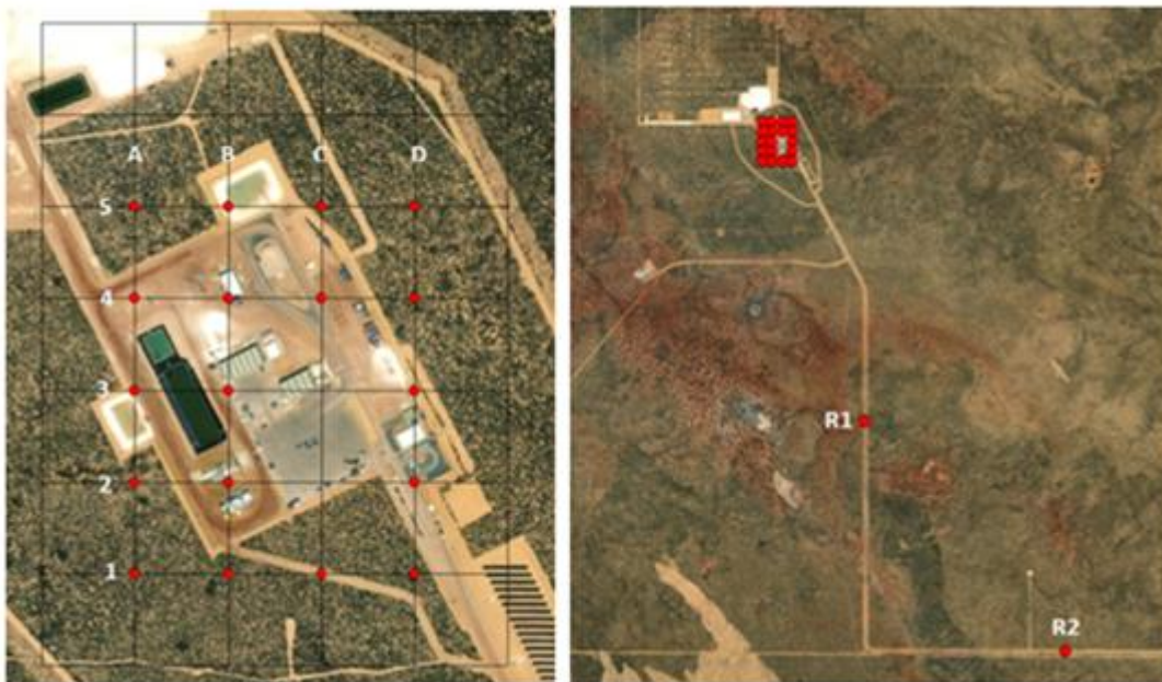
Figure 2-1: 400m x 500m soil sampling grid over the Sandy Ridge Infrastructure Area. Red dots indicate soil sampling locations. Two additional access road sampling locations (R1 and R2) are shown to the right.
