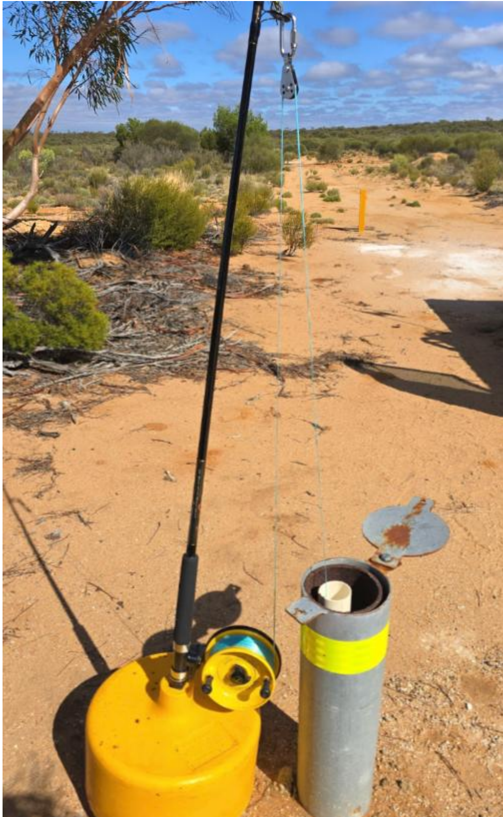
Figure 5-1: Groundwater sampling equipment. Recent improvements include stabilising base, and a pulley to reduce friction while lifting water samples.
