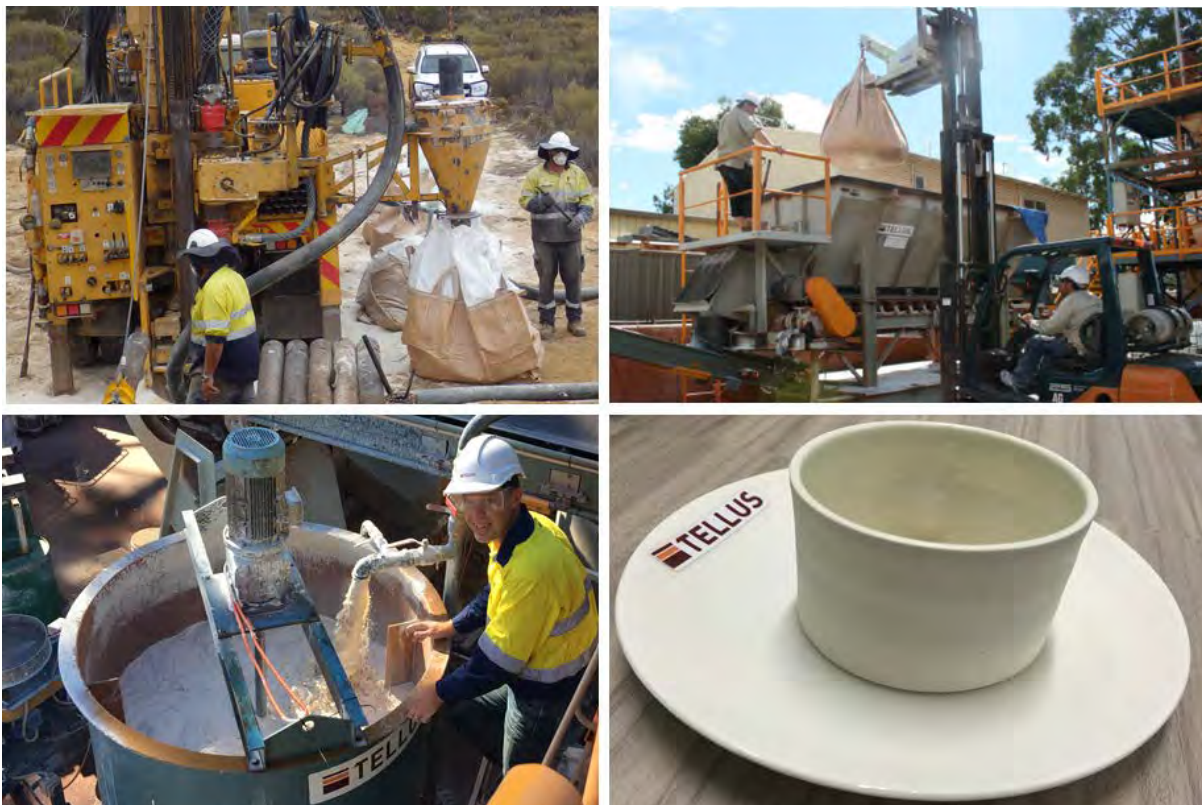
Plate 1-1 Process from the proponents drilling, to bulk pilot, to producing ceramic grade products
