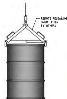
TYPICAL DRUM LIFTING ARRANGEMENT SCALE 1:10
