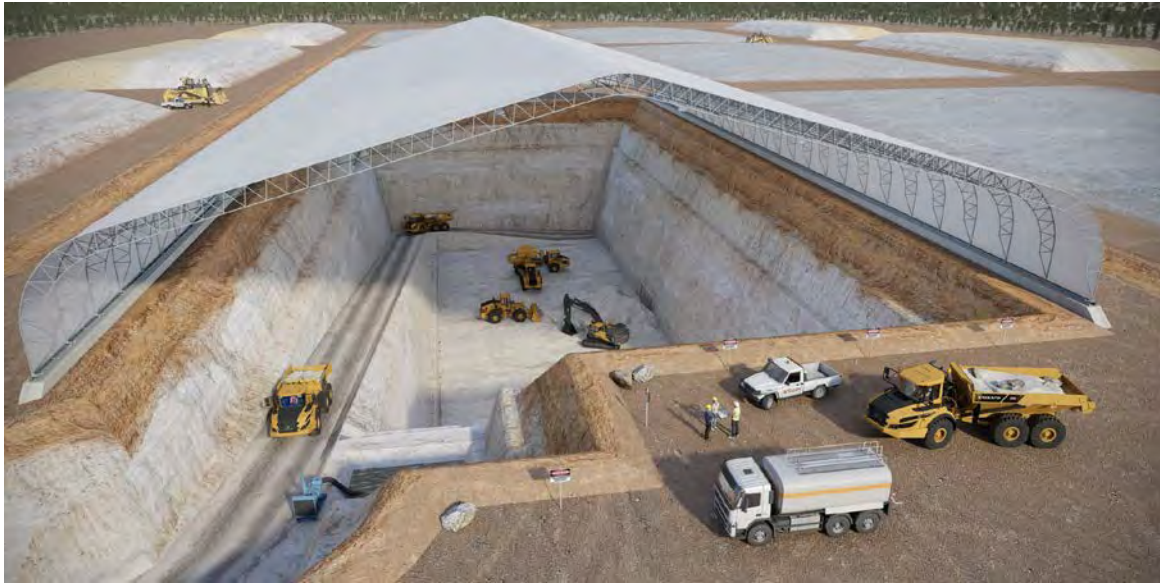
Conceptual view of pit being mined. Roof canopy is erected at the later stages of kaolin mining, prior to waste emplacement to prevent rainfall from entering the waste cell.
